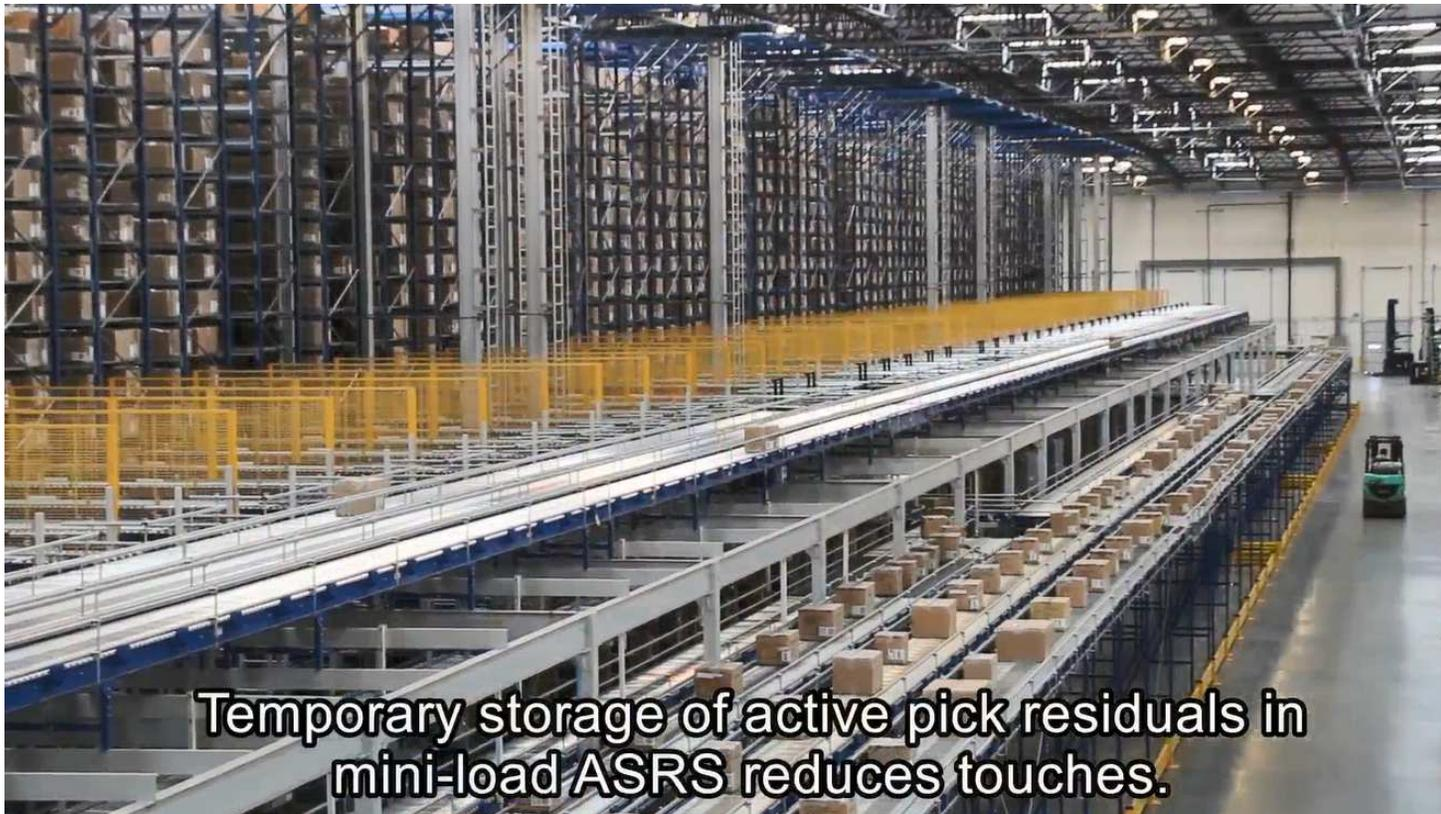
**Temporary storage of active pick residuals in mini-load ASRS reduces touches.**
